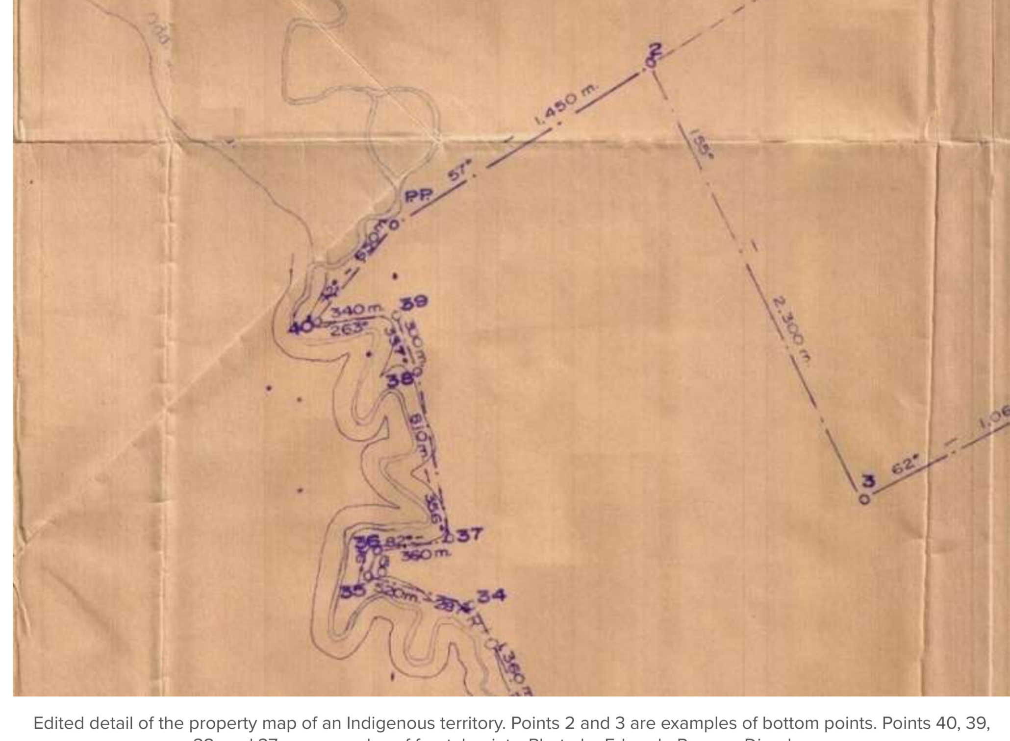
Edited detail of the property map of an Indigenous territory. Points 2 and 3 are examples of bottom points. Points 40, 39, 38, and 37 are examples of frontal points. Photo by Eduardo Romero Dianderas.
