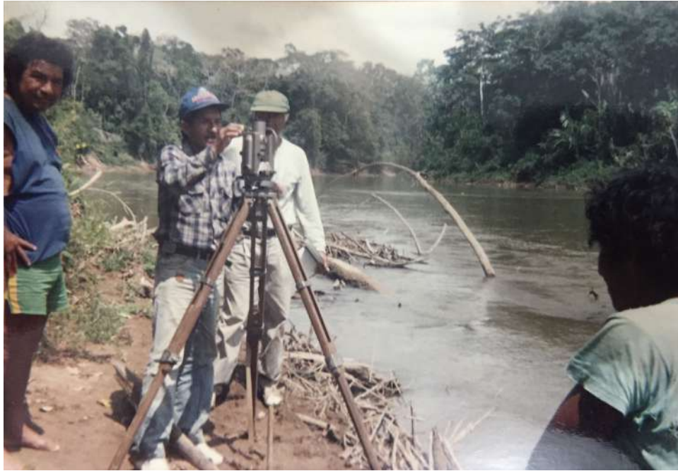
FIGURE 2 Working in the Peruvian Amazon, an engineer ( ingeniero ) measures an Indigenous property polygon on the ground with classical topography, before GPS technologies were available. Undated photograph from the mid-1990s. (Centro para el Desarrollo del Indígena Amazónico) [This figure appears in color in the online issue]
